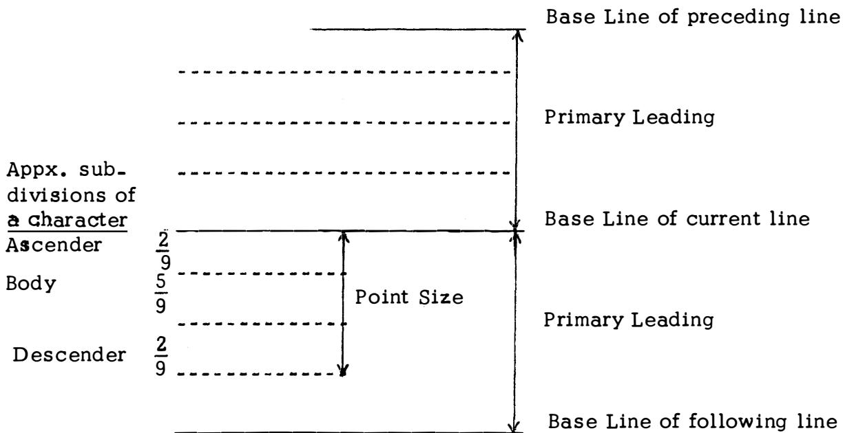
Note : The base line for a character is conventionally at the foot of the ascender i.e.  $\frac{2}{9}$  down from the top of a tall character such as h. The convention used here, namely putting the base line at the top of the ascender conforms with the current setting of the CSIR machine.
