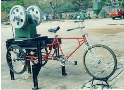
Figure 7: Bicycle pedaled crusher
