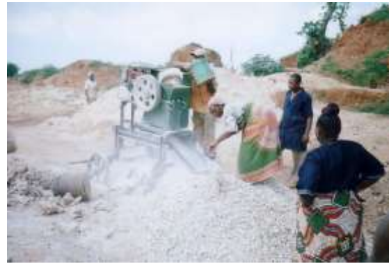
Figure 8: Diesel engine operated crusher
